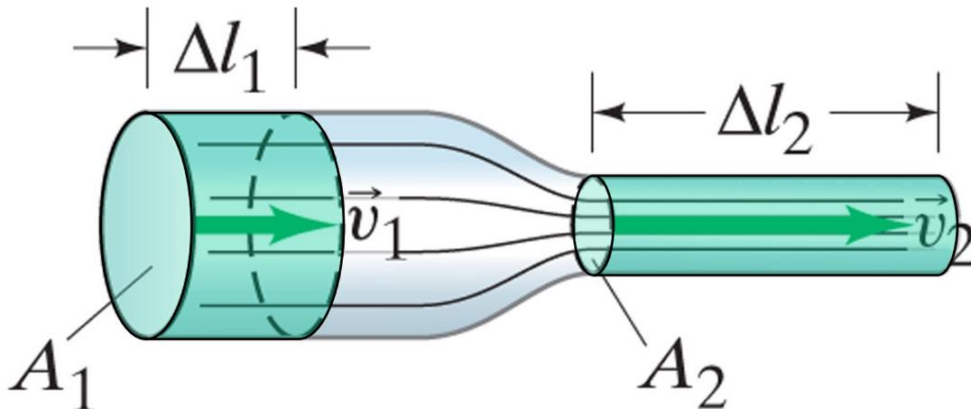
$$\frac{\Delta m_1}{\Delta t} = \frac{\Delta m_2}{\Delta t} \rightarrow \rho_1 A_1 v_1 = \rho_2 A_2 v_2$$
